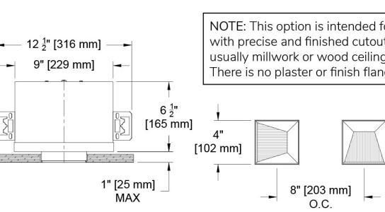
NOTE: This option is intended for use with precise and finished cutouts - usually millwork or wood ceilings. There is no plaster or finish flange.
